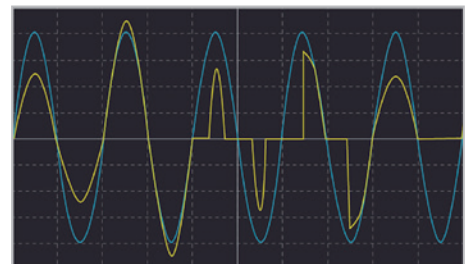
List Mode Load Waveform Composed of Multiple Current Types
