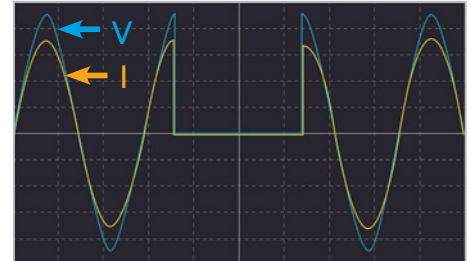
Voltage Interruption Load Test in CR Mode
