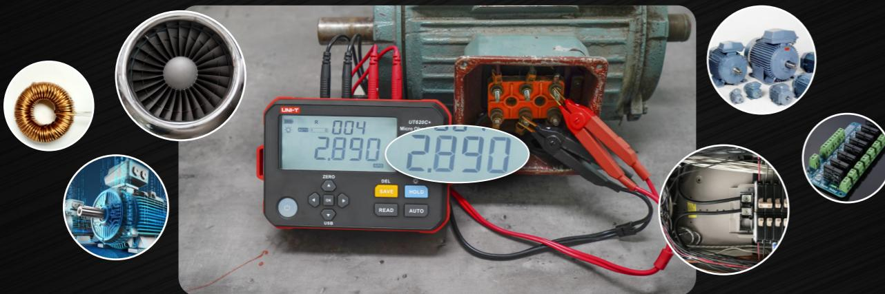
Measuring the resistance of all kinds of wires, switches, connectors, contactors, fuses, coils, transformer windings, metal riveting, and so on.
